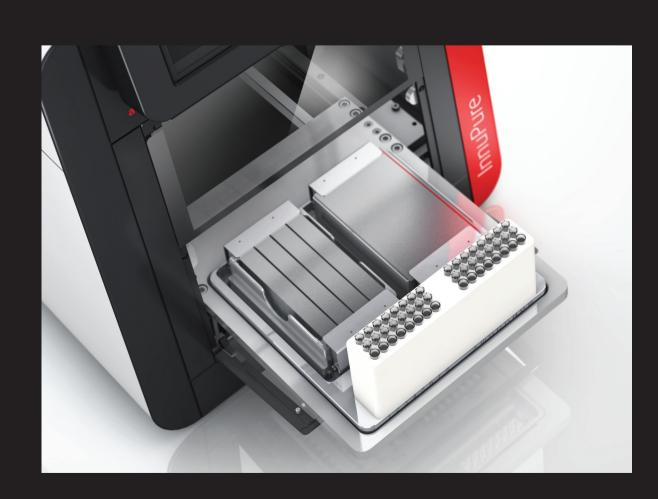
InnuPure® C16 touch combines highly precise liquid handling with automated extraction of high-quality nucleic acids.
